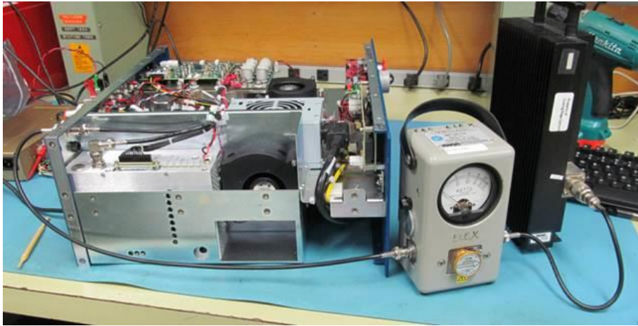
Figure 2 Byrd Watt Meter and 50 ohm RF Load Connected to RF OUT 1
