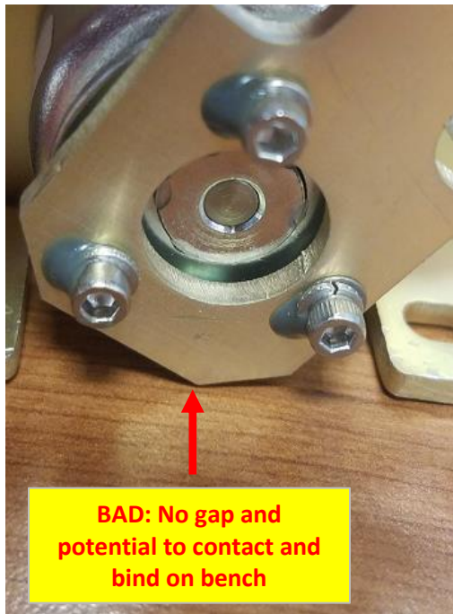
Figure 6: No Gap Causing Interference
