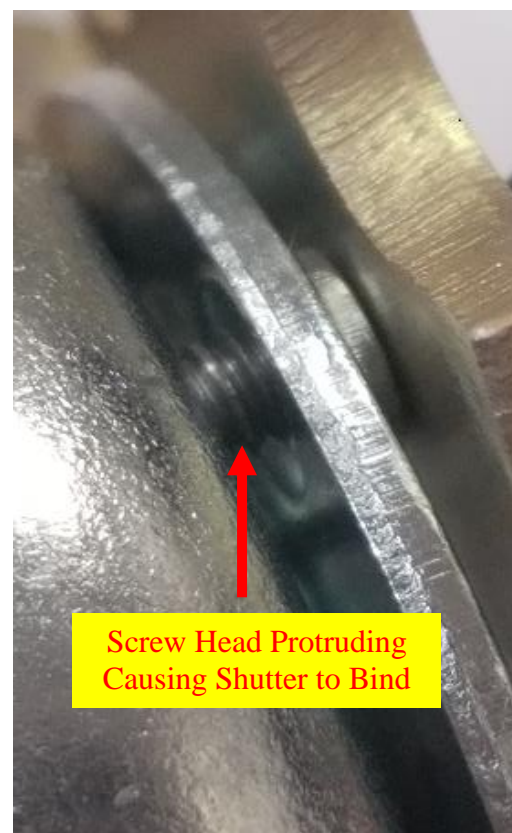
Figure 2: Protruding Screw – Close Up
