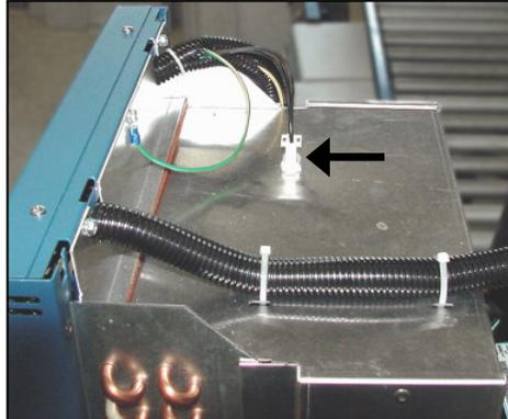
Figure L – Fan motor mounting nuts
