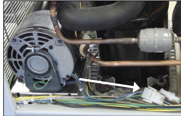
7. Slide pump/bracket assembly out of the right side (when facing the rear) of the chiller. If replacing the motor in a chiller with a positive displacement pump, it will also be necessary to remove the pump head (see Section 3.6)
