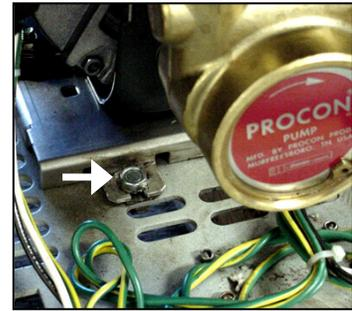
6. Unplug pump wiring quick-disconnect plug (see Figure G)
