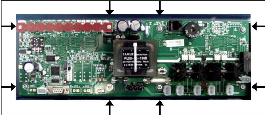
8. Remove circuit board. Be sure to observe all ESD precautions when handling both the defective and replacement PC boards. Install new board by following previous steps in reverse.
