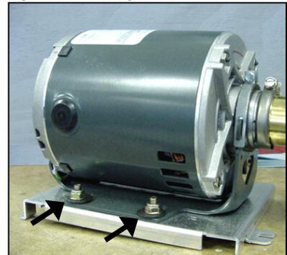
9. Mount new motor onto mounting bracket and install by following the previous steps in reverse.
